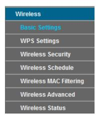
There are seven submenus under the Wireless menu: Basic Settings, WPS Settings, Wireless Security, Wireless Schedule, Wireless MAC Filtering, Wireless Advanced and Wireless Status. Click any of them, and you will be able to configure the corresponding function.
