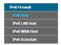
There are four submenus under the IPv6 Firewall menu: IPv6 Rule, IPv6 LAN Host, IPv6 WAN Host and IPv6 Schedule. Click any of them, and you will be able to configure the corresponding function.
