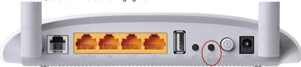
You can also keep the default WPS Status as **Enabled** and click the **Add device** button in Figure 4-43, then Choose "**Press the button of the new device in two minutes**" and click **Connect**. (Shown below)
