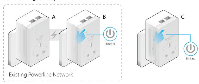
Powerline adapter A and Powerline adapter B form a HomeplugAV Network, Powerline adapter C wants to join this network.
