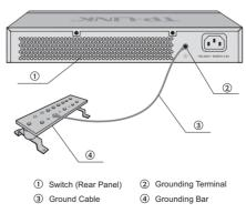
Figure 3-1 Connecting to the Grounding Bar
