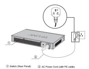
Figure 3-2 Connecting to the Ground
