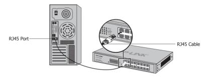
Figure 4-1 Connecting the RJ45 Port
