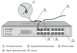
Figure 3-4 Lighting Arrester Connection
