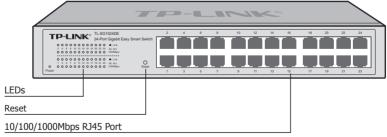
Figure 1-2 Front Panel of TL-SG1024DE
