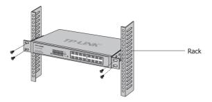
Figure 2-3 Rack Installation
