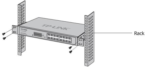
Figure 2-3 Rack Installation
