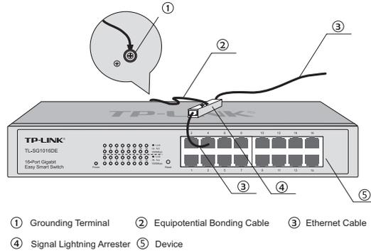
Figure 3-4 Lighting Arrester Connection
