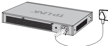
Figure 4-2 Connecting to Power Supply
