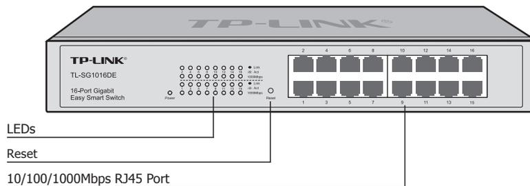
Figure 1-1 Front Panel of TL-SG1016DE
