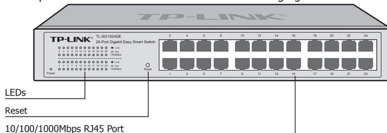
Figure 1-2 Front Panel of TL-SG1024DE
