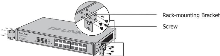
Figure 2-2 Bracket Installation
