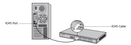
Figure 4-1 Connecting the RJ45 Port
