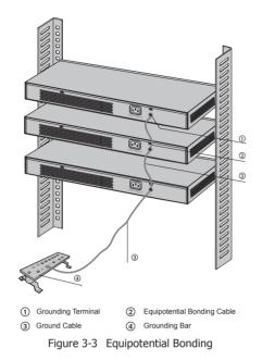
The figure below illustrates how to practice equipotential bonding in a network.
