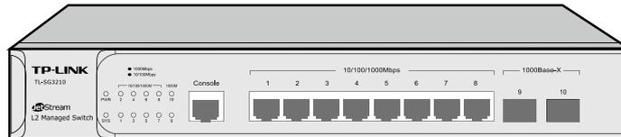
Figure 2-1 Front Panel of TL-SG3210
