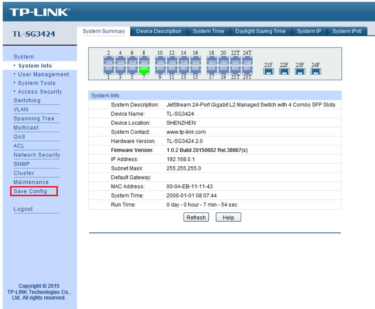
The screenshot displays the TP-LINK web management interface for a TL-SG3424 switch. The top navigation bar includes tabs for System Summary, Device Description, System Time, Daylight Saving Time, System IP, and System IPv6. The left sidebar lists various configuration categories, with 'Save Config' highlighted in red. The main content area features a port status diagram showing 24 ports (1-24) and 4 SFP slots (21F-24F). Below this is a 'System Info' table with the following data:
