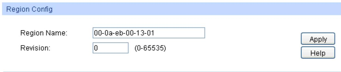
The screenshot shows a web interface for configuring an MSTP region. At the top, there is a blue header bar with the text "Region Config". Below this, there are two rows of configuration fields. The first row is labeled "Region Name:" and has a text input field containing "00-0a-eb-00-13-01". The second row is labeled "Revision:" and has a numeric input field containing "0", followed by the text "(0-65535)". To the right of these fields are two buttons: "Apply" and "Help".
