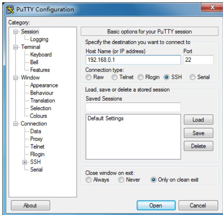
2. Click the **Open** button in the above figure to log on to the switch. Enter the login user name and password, and then you can continue to configure the switch.
