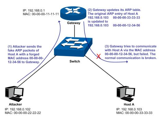
Figure 12-10 ARP Attack – Cheating Gateway
