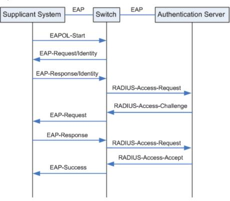
Figure 12-18 EAP-MD5 Authentication Procedure
