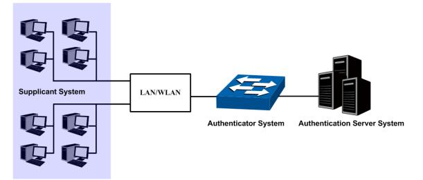
Figure 12-17 Architecture of 802.1X authentication
