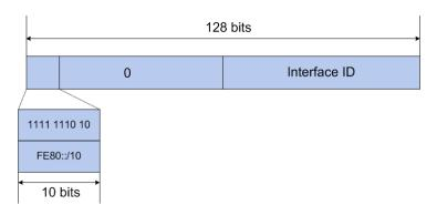
Figure 4-9 Link-local Address Format
