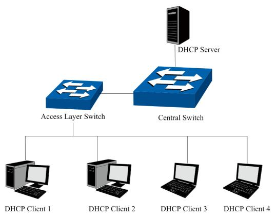
Figure 12-5 Network diagram for DHCP-snooping implementation
