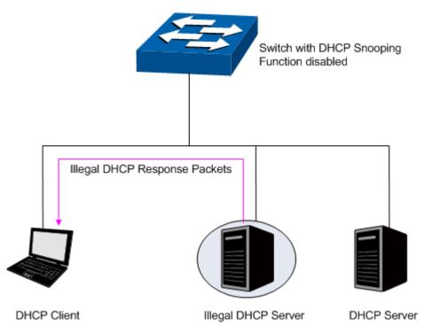
Figure 12-7 DHCP Cheating Attack Implementation Procedure
