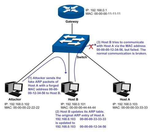
Figure 12-11 ARP Attack – Cheating Terminal Hosts
