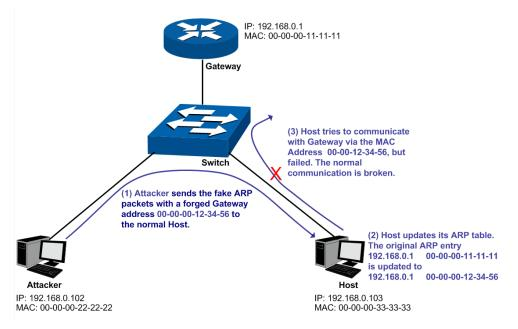
Figure 12-9 ARP Attack - Imitating Gateway
