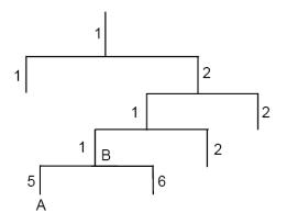
Figure 13-2 Architecture of the MIB tree
