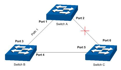
Figure 7-1 Basic STP diagram
