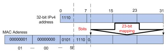
Figure 8-2 Mapping relationship between multicast IPv4 address and multicast MAC address
