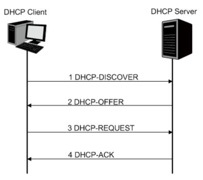
Figure 12-6 Interaction between a DHCP client and a DHCP server
