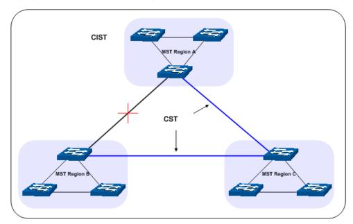
Figure 7-2 Basic MSTP diagram
