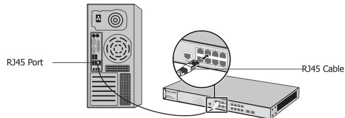
Figure 4-1 Connecting the RJ45 Port
