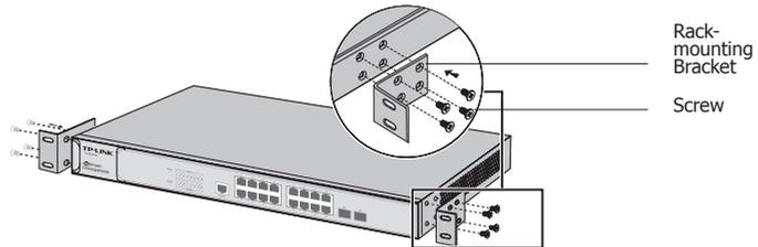
Figure 2-2 Bracket Installation
