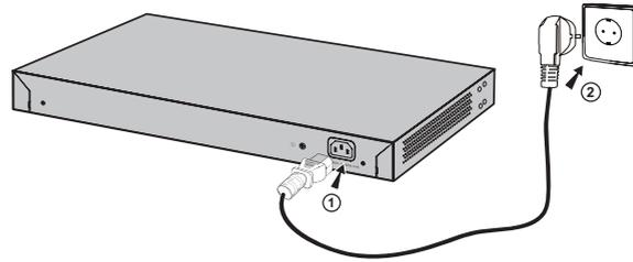
Figure 4-4 Connecting to Power Supply
