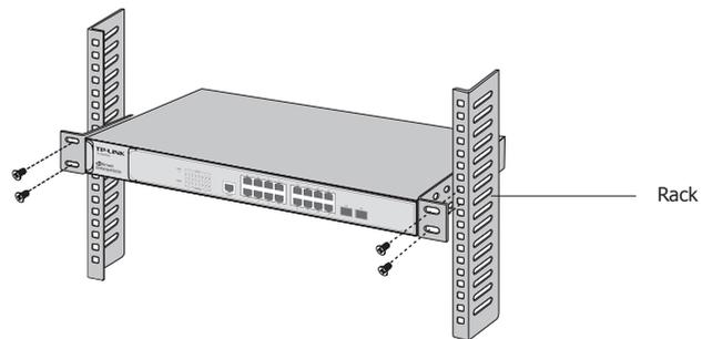
Figure 2-3 Rack Installation
