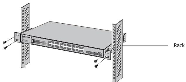
Figure 2-3 Rack Installation
