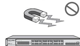
Electronic elements including capacitance and inductance on the device can be affected by external interferences, such as conducted emission by capacitance coupling, inductance coupling, and impedance coupling. To decrease the interferences, please make sure to take the following measures:
