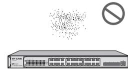
The dust accumulated on the Switch can be absorbed by static electricity and result in poor contact of metal contact points. Some measures have been taken for the device to prevent static electricity, but too strong static electricity can cause deadly damage to the electronic elements on the internal circuit board. To avoid the effect of static electricity on the operation of the Switch, please attach much importance to the following items:
