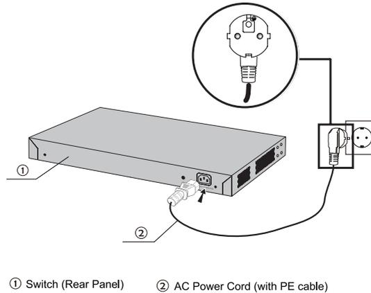
Figure 3-2 Connecting to the Ground
