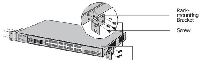
Figure 2-2 Bracket Installation
