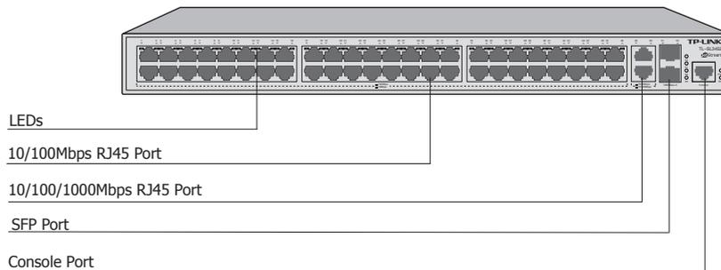
Figure 1-2 Front Panel of TL-SL3452
