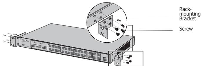
Figure 2-2 Bracket Installation
