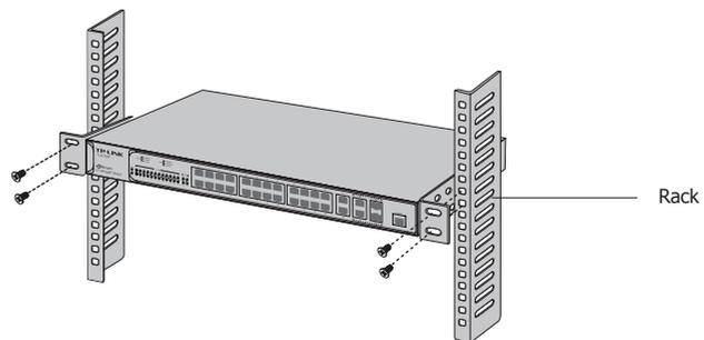
Figure 2-3 Rack Installation
