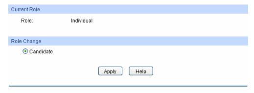
Figure 16-16 Cluster Configuration for Individual Switch
