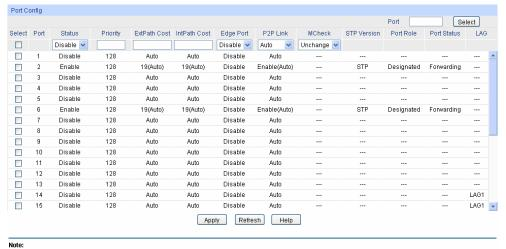
If the Path Cost of a port is set to 0, it will alter automatically according to the port's link speed.
