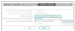
c. Fill in the Wi-Fi Password of your main Router/AP. The TL-WA850RE's Wi-Fi network name (SSID) can be copied from your main Router/AP name (TP-LINK\_XXX) OR BE CUSTOMIZED A NEW ONE (TP-LINK\_XXX\_EXT).
