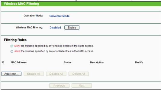
Figure 4-15 Wireless MAC address Filtering
