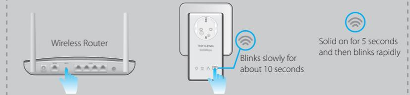
**Note:** If the Wi-Fi LED still blinks slowly for longer than 30 seconds, unplug the extender and plug it back in, then try again. Or use "Customize the Extender's Wi-Fi Settings" on the back instead.
