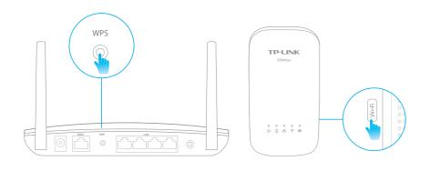
3. When the 2.4GHz Wi-Fi LED 중 and 5GHz Wi-Fi LED 중 on the extender blink quickly for 3 seconds and then stay on, use the router's SSID and password to join the Wi-Fi network.
