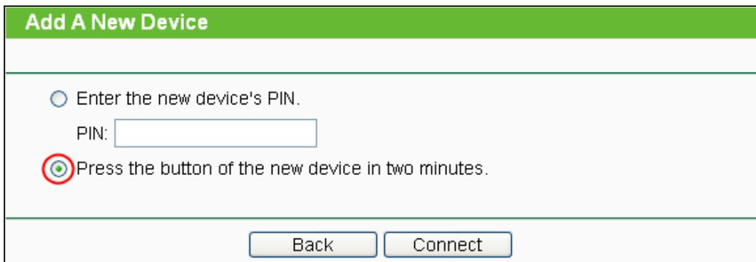
Step 2: Choose “**Press the button of the new device in two minutes**” and click **Connect**.
