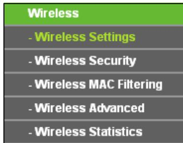
There are five submenus under the Wireless menu: **Wireless Settings**, **Wireless Security**, **Wireless MAC Filtering**, **Wireless Advanced** and **Wireless Statistics**. Click any of them, and you will be able to configure the corresponding function.
