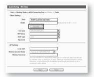
3 The target network's SSID and BSSID will automatically fill the relevent wireless setting boxes. Select the **Key type** and enter the **Password**. Click "**Next**" and then "**Reboot**".
