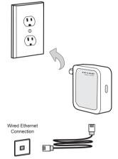
If you are connecting the TL-WR710N directly to your **cable modem**, you must first power reset the modem and **wait until its ONLINE LED is solid**. Then use an ethernet cable to connect to your modem via the **LAN/WAN** port on the TL-WR710N.
