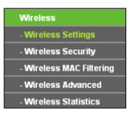
There are five submenus under the Wireless menu: Wireless Settings, Wireless Security, MAC Filtering, Wireless Advanced and Wireless Statistics. Click it, and you will be able to configure the corresponding function.
