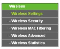
There are five submenus under the Wireless menu: Wireless Settings, Wireless Security, Wireless MAC Filtering, Wireless Advanced and Wireless Statistics. Click any of them, and you will be able to configure the corresponding function.
