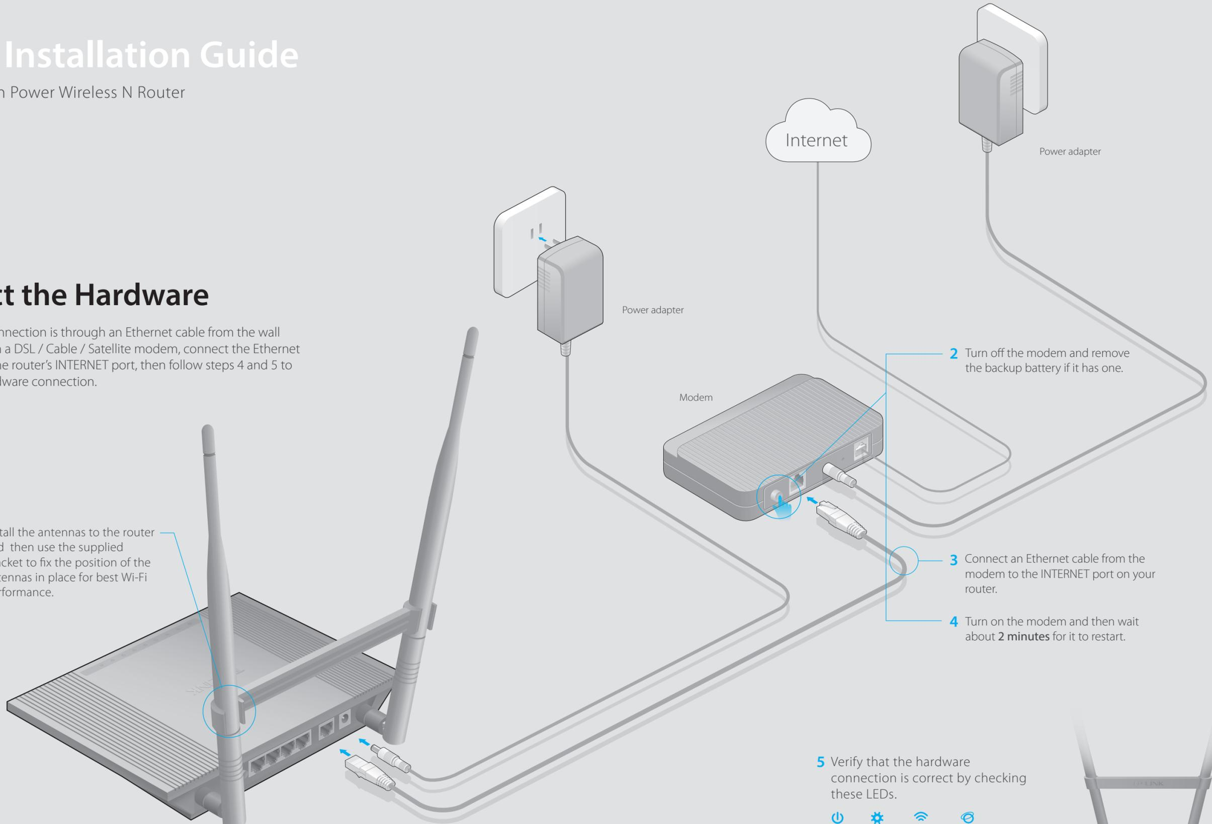
**2** Turn off the modem and remove the backup battery if it has one.
