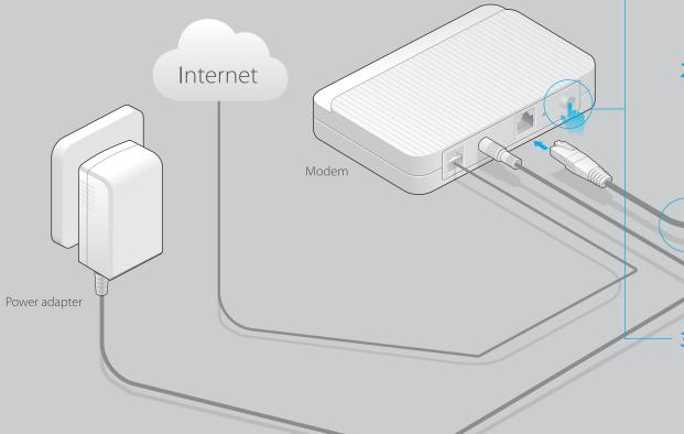
Turn off the modem, and remove the backup battery if it has one.
