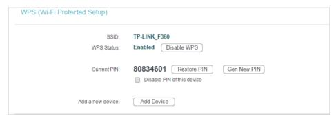
2. Enter the router's current PIN on your client device to join the router's Wi-Fi network.
