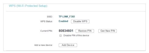
2. Enter the router's current PIN on your client device to join the router's Wi-Fi network.
