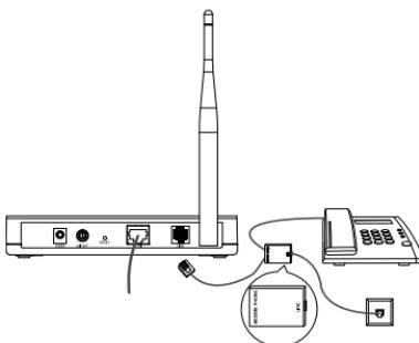
**Note** If no telephone is needed, please connect the LINE port of the Modem Router to the wall jack using the telephone line directly.
