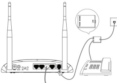
**Note** If no telephone is needed, please connect the ADSL port of the Router to the wall jack using the telephone line directly.
