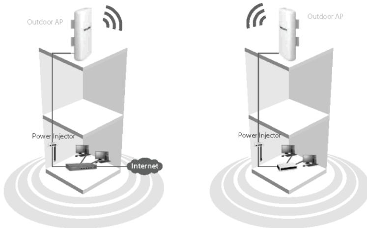
**Note** The typical connection for TL-WA5210G is shown as above. Please make sure that the two CPEs are placed face to face, otherwise the wireless signal strength might be weak. Here shows several incorrect examples.
