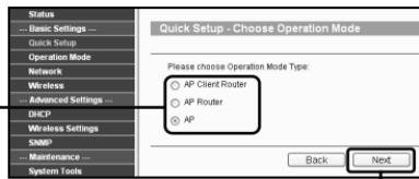
**Note** The AP supports three operation mode types: **AP Client Router**, **AP Router** and **AP**.
