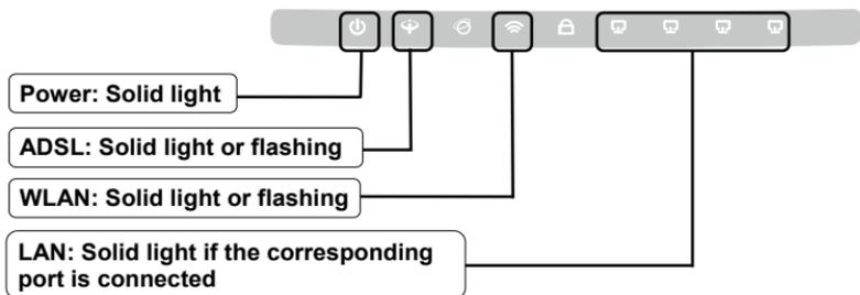
**Note** If the LEDs display abnormally, please check to see if all the cable connectors (power adapter, phone line and Ethernet cable) are well connected to your device. With the phone line well connected, if the ADSL LED turns off after flashing, please contact your ISP to ensure that your internet connection is active.
