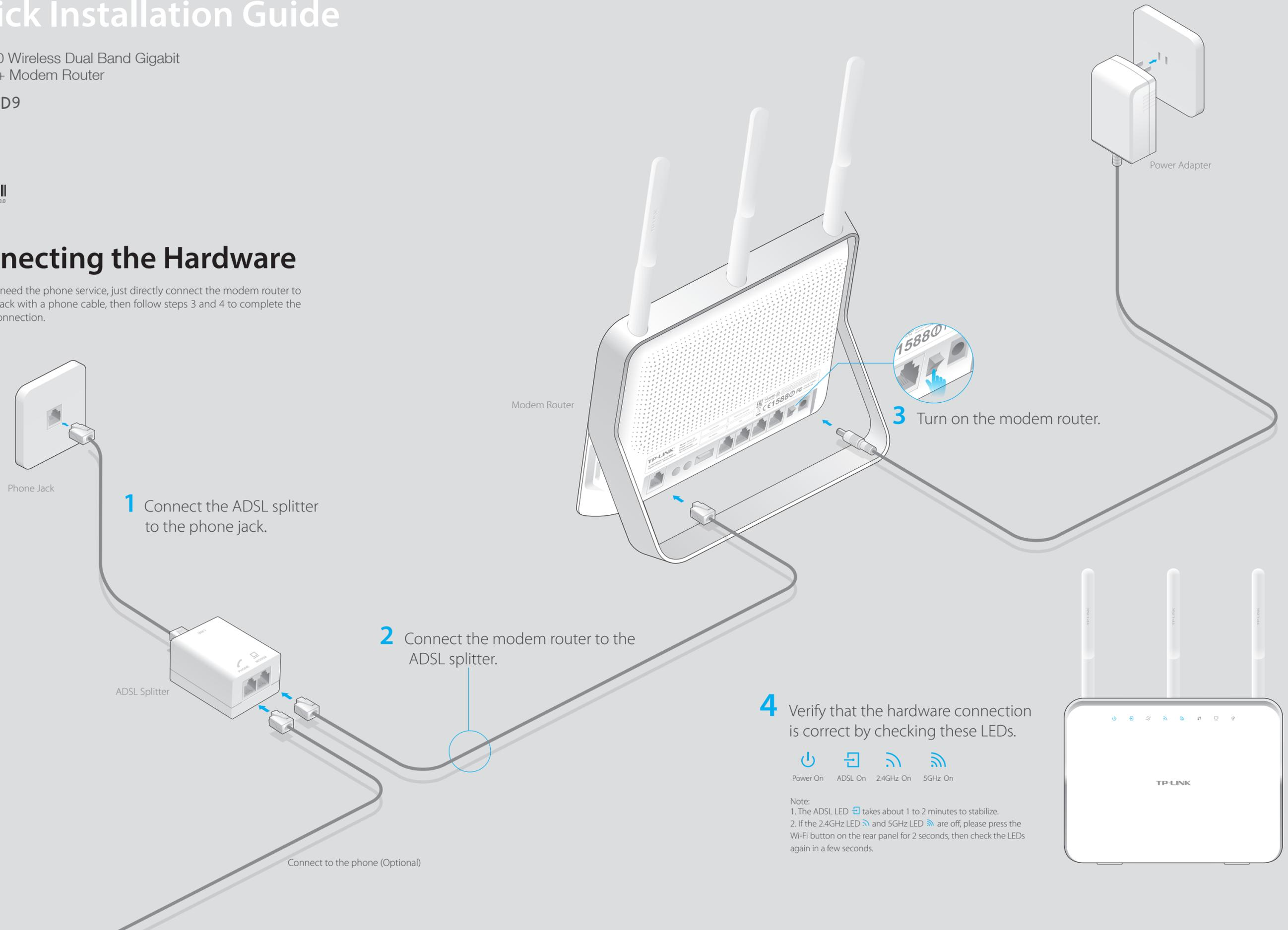
4 Verify that the hardware connection is correct by checking these LEDs.
