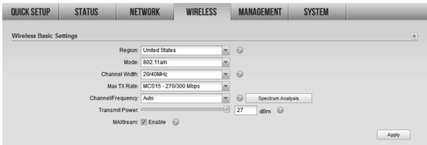
Pharos MAXstream is a non-standard Wi-Fi protocol that is only compatible with TP-LINK's Pharos series products. Please notice that you will not be able to connect other Wi-Fi devices to an AP with MAXstream enabled.
