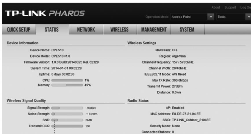
Adjust the direction of the CPE until the device reaches the highest SNR.
