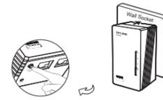
**4** Place the extender in your desired location. The extender will automatically synchronize wireless settings with the router whenever the router's wireless settings are changed.
