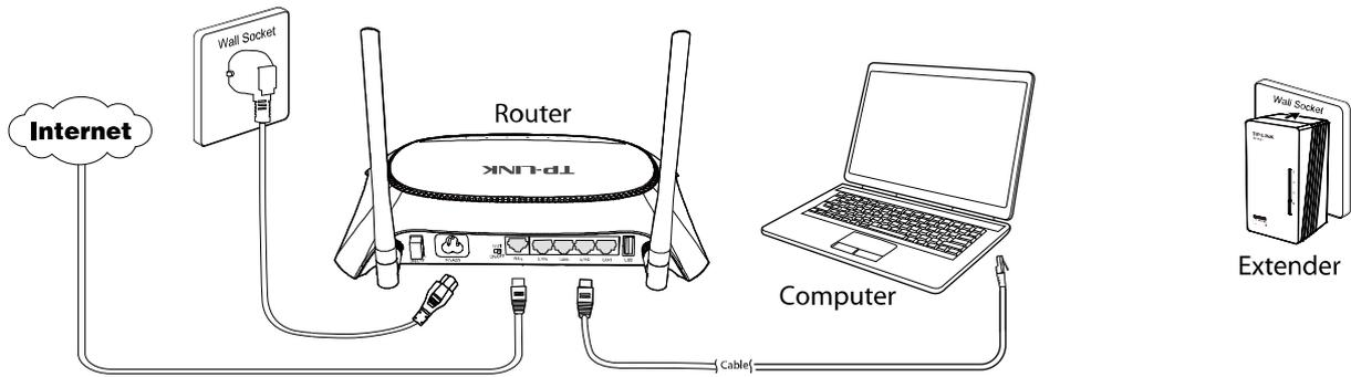
Figure 2-1 Hardware connection
