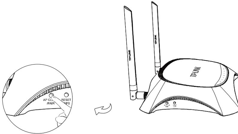
3. Press the AP CLONE/PAIR button on the extender's bottom and the extender's Power LED will blink quickly. In about 20 seconds, both Powerline LEDs will be solid on, indicating that the router and the extender have formed a powerline network. Then both Power LEDs will be solid on, indicating that the AP clone process is completed.
