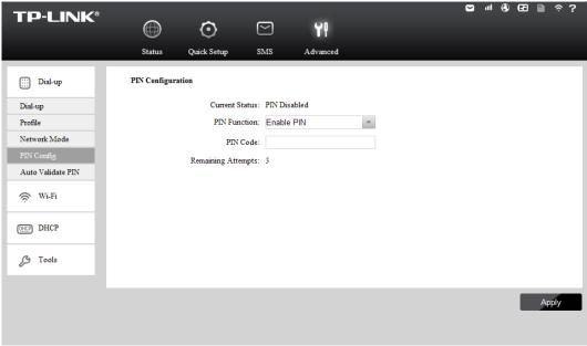
Figure 4-16 PIN Configuration
