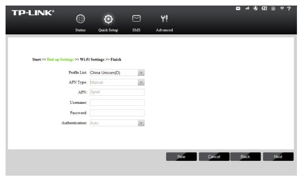
Figure 3-3 Quick Setup – Dial-up Settings
