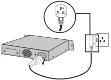
Figure 3-4 Connecting to Power Supply
