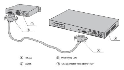
Figure 3-3 Connecting to the Powered Switch
