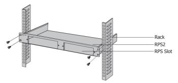
Figure 2-2 Install the RPS2 to a standard rack
