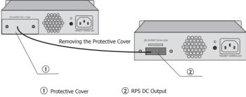
Figure 3-2 Removing the RPS Protective Cover
