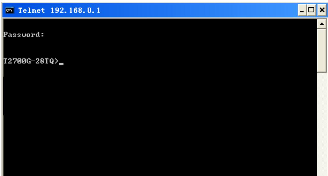
Figure 1-14 Enter into the User EXEC Mode
