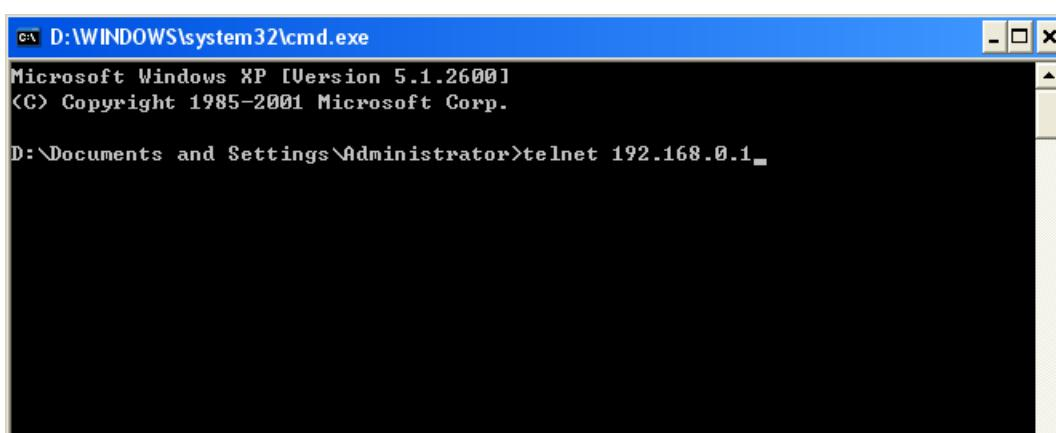
Figure 1-9 Connecting to the Switch
