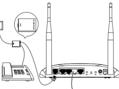
**Note** If no telephone is needed, please connect the ADSL port of the modem router to the wall jack using the telephone line directly.
