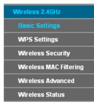
There are six submenus under the Wireless menu: **Basic Settings**, **WPS Settings**, **Wireless Security**, **Wireless MAC Filtering**, **Wireless Advanced** and **Wireless Status**. Click any of them, and you will be able to configure the corresponding function.
