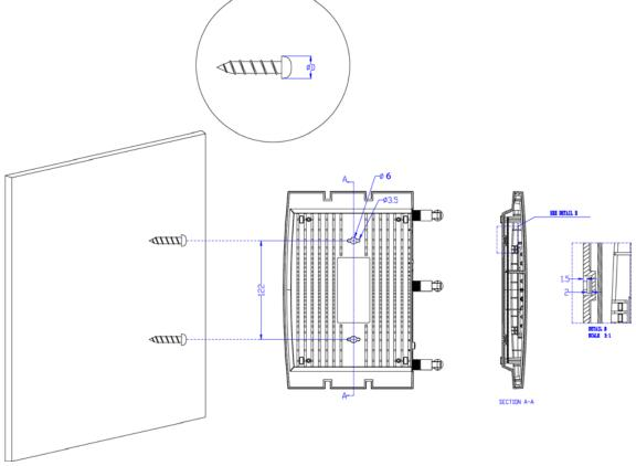
Figure 2-1 Wall-mount install
