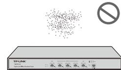
The dust accumulated on the router can be absorbed by static electricity and result in poor contact of metal contact points. Some measures have been taken for the device to prevent static electricity, but too strong static electricity can cause deadly damage to the electronic elements on the internal circuit board. To avoid the effect of static electricity on the operation of the router, please attach much importance to the following items:
