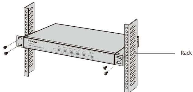
Figure 2-3 Rack Installation
