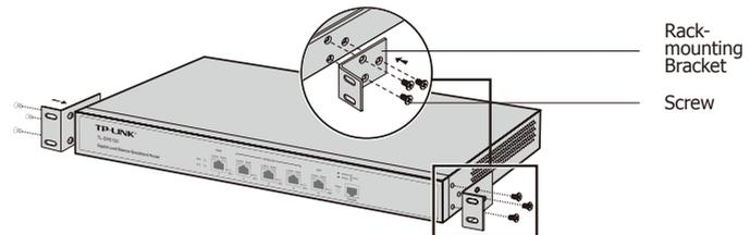
Figure 2-2 Bracket Installation
