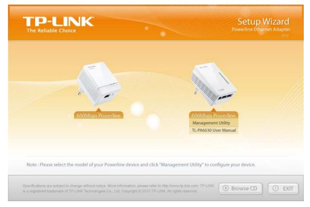
Step 2: Choose TL-PA6030, select **600Mbps Powerline** and click **Management Utility**, and then the program installation process will carry out and copy all the necessary files to your system.
