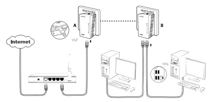
Create a secured powerline network using the Pair button:
