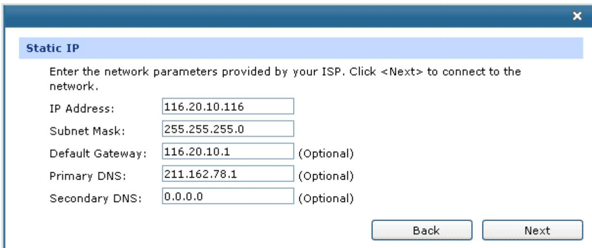
Figure 3-15 WAN Connection Type - Static IP
