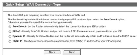
**Auto-Detect:** If Auto-Detect is chosen, the router will detect the connection type provided by your ISP automatically.
