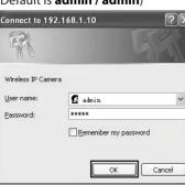
3 When accessing the IP Camera for the first time, a yellow information bar will appear below the address bar. Click the information bar, and select "Install ActiveX Control..."
