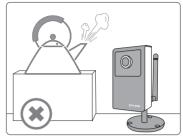
• Do not place the Camera where there are high temperatures such as near an oven.
