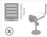
Do not place the Camera near devices that emit radio waves, such as mobile phones.
