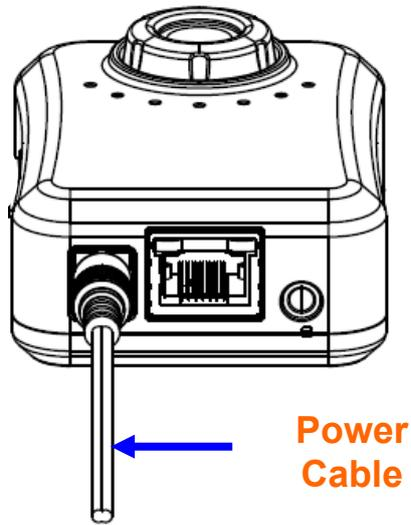
Once you have installed the camera well and powered it on, the Power LED (orange) will turn on later. Once the Power LED turned on, it means the system is booting up successfully. Furthermore, if you have a proper network connection, and access to the camera, the LAN LED (green) will flash green under wired mode.
