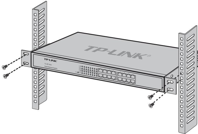
Figure 1-2 Fasten the Switch in the Rack
