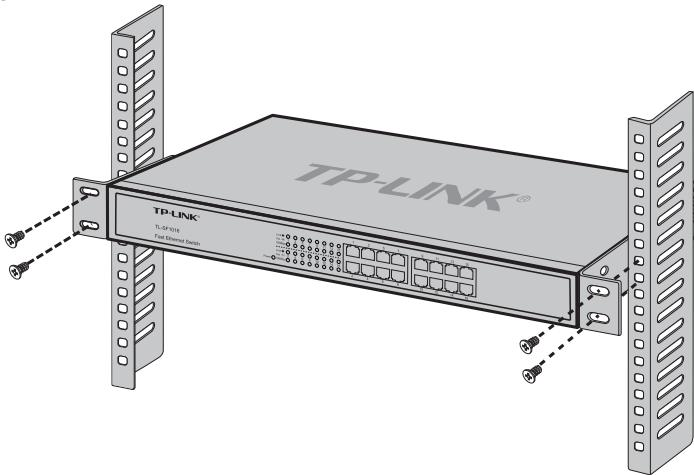
Figure 3-3 Mounting Switch
