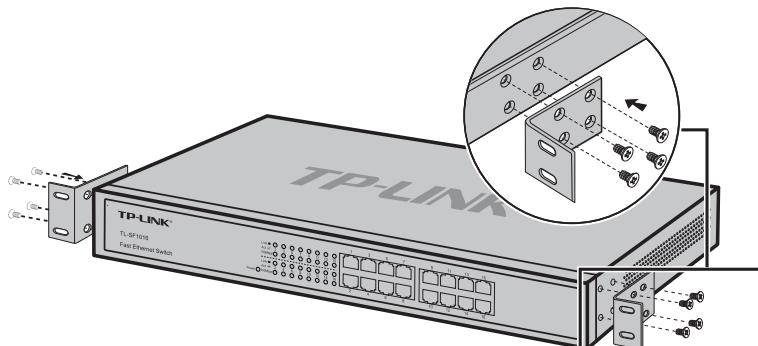
Figure 1-1 Rivet the "L" brackets onto the Switch
