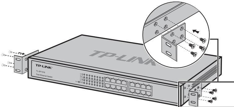
Figure 3-2 Attaching Brackets
