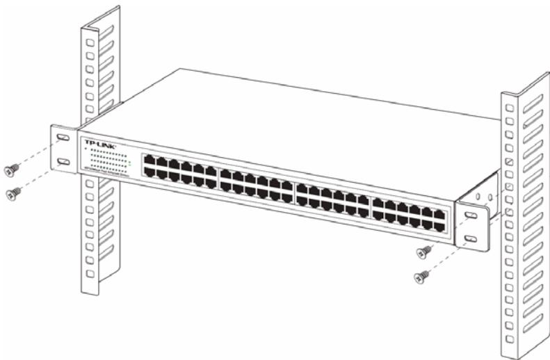
Figur 2-2 Sätt fast switchen i stativet
