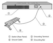
Figure 3-1 Connecting to the Grounding Bar
