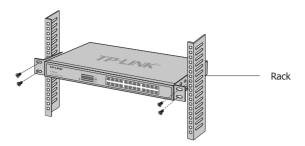
Figure 2-3 Rack Installation
