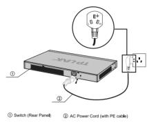
Figure 3-2 Connecting to the Ground
