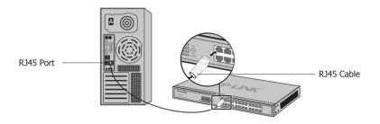
Figure 4-1 Connecting the RJ45 Port
