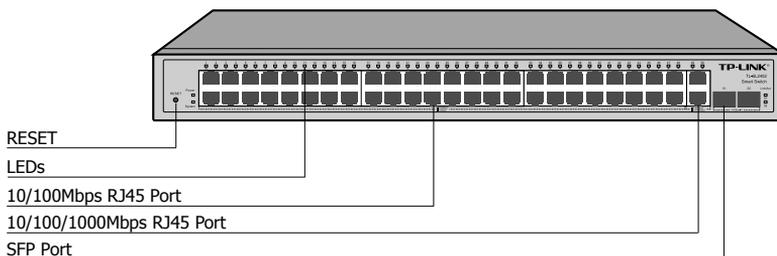
Figure 1-4 Front Panel of TL-SL2452
