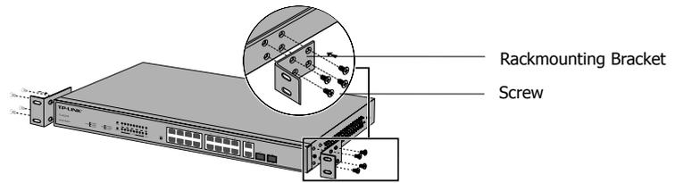
Figure 2-2 Bracket Installation
