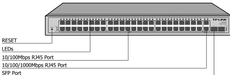
Figure 1-4 Front Panel of TL-SL2452
