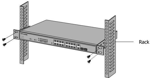
Figure 2-3 Rack Installation
