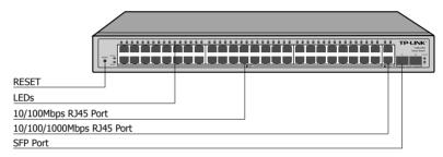
Figure 1-4 Front Panel of TL-SL2452
