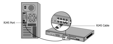
Figure 4-1 Connecting the RJ45 Port
