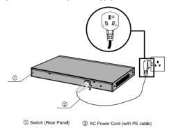
Figure 3-2 Connecting to the Ground
