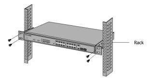
Figure 2-3 Rack Installation
