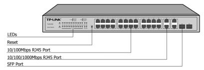
Figure 1-3 Front Panel of TL-SL2428
