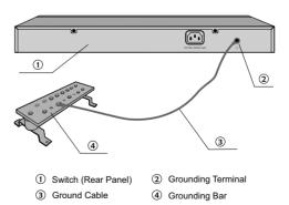
Figure 3-1 Connecting to the Grounding Bar
