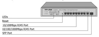
Figure 1-1 Front Panel of TL-SL2210
