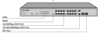
Figure 1-2 Front Panel of TL-SL2218
