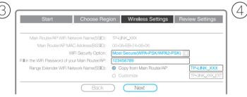
Enter your router's WiFi password for connecting to the router. For Range Extender's wireless network name (SSID), you can either copy it from the router or create a new one.
