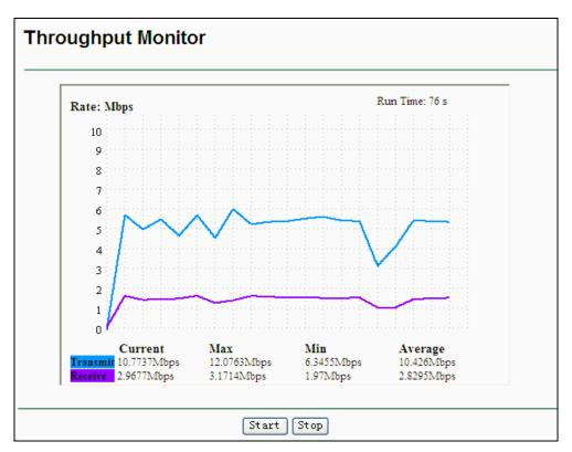
Figure 4-19 Throughput Monitor
