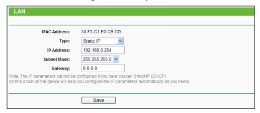
Figure 4-7 LAN - Static IP
