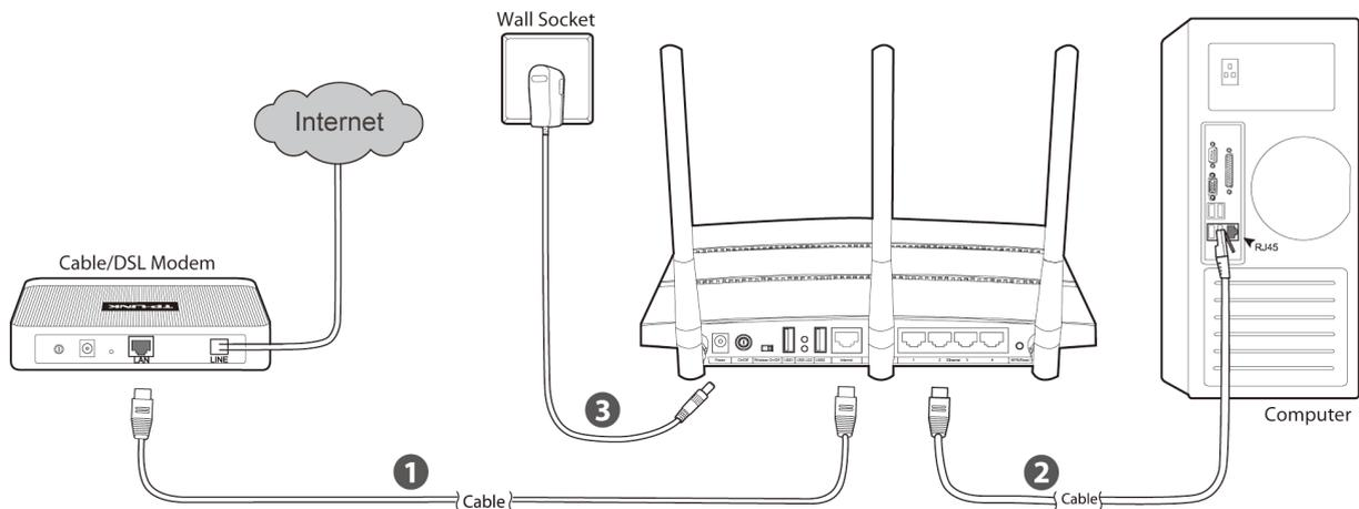
Figure 2-1 Hardware Installation
