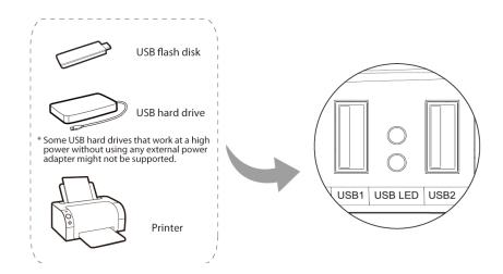
Figure 2-2 USB Installation
