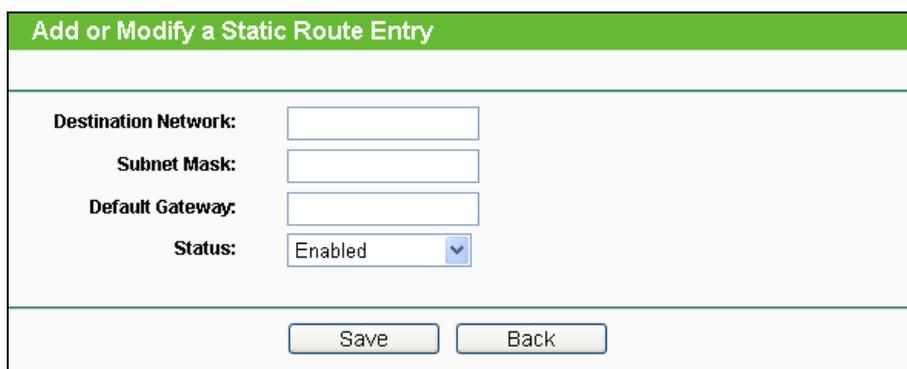
Figure 4-97 Add or Modify a Static Route Entry
