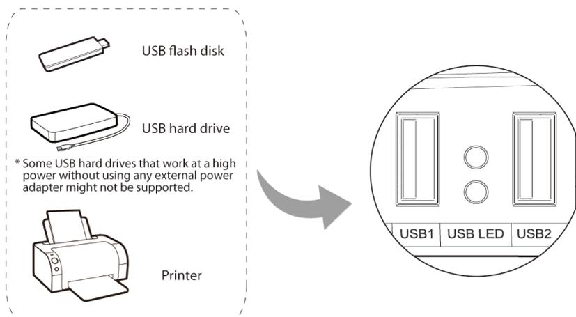
Figure 2-2 USB Installation
