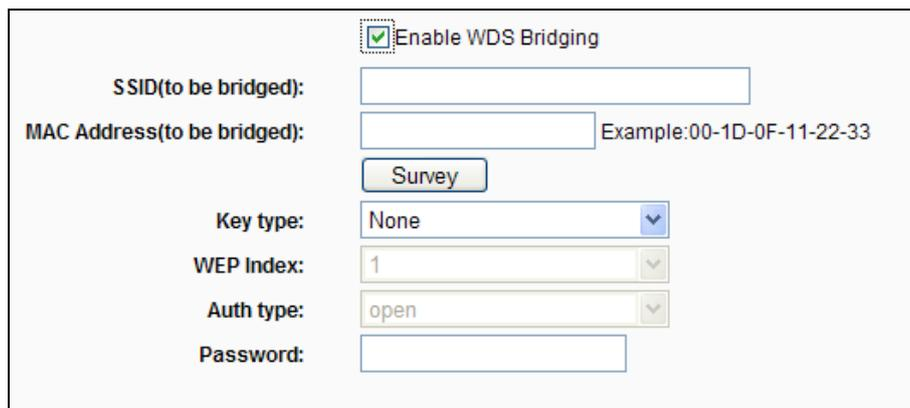
The screenshot shows the WDS (Wireless Distribution System) configuration interface. At the top, the checkbox for 'Enable WDS Bridging' is checked. Below this, there are several input fields and dropdown menus:
