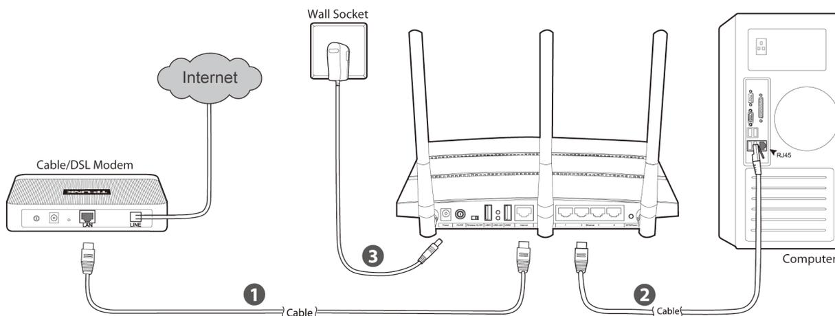
Figure 2-1 Hardware Installation
