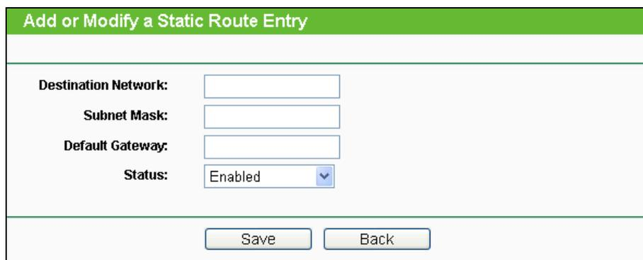
Figure 4-93 Add or Modify a Static Route Entry
