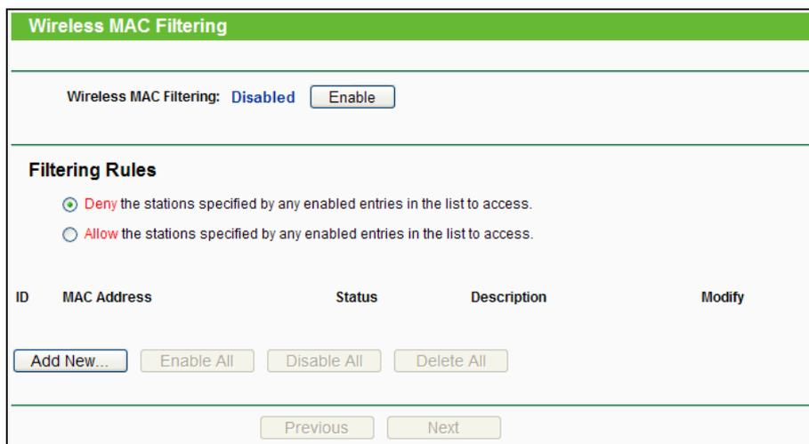
Figure 4-24 Wireless MAC Filtering
