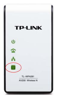
Step 2: Within two minutes, press and hold the QSS button of the adapter directly for 2 or 3 seconds. (QSS, also called WPS, is used by our company on the wireless adapter.)
