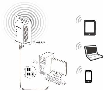
As soon as the powerline devices are connected following the steps above, a usable powerline network is available.
